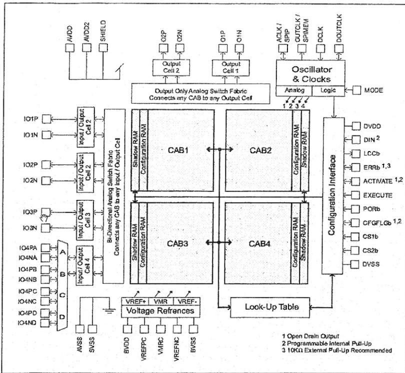
Fig. 8. The inner structure of AN221E04 FPAA's (Anadigm)
