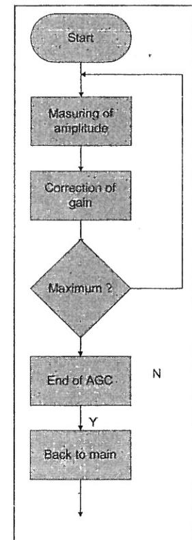
Fig. 10. The Automatically gain correction
